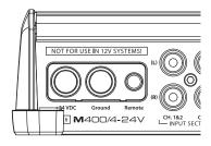
The M400/4-24V's "+24 VDC" and "Ground" connections are designed to accept up to 4 AWG power wire. 8 AWG is the required wire size for this amplifier.
