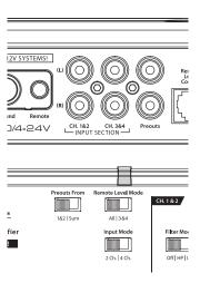
If you wish to send four discrete channels into the M400/4-24V, simply use all four inputs and set the "Input Mode" switch in the "4 Ch." position.
