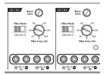
1) "Filter Mode" Control: The M400/4-24V employs a 12dB per octave filter for each pair of channels (one filter for channels 1&2, another filter for channels 3&4 and a third filter for channels 5&6). Each of these filters can be configured independently into one of two filter
