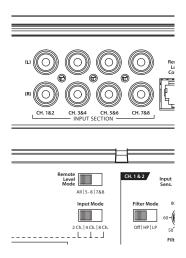
If you wish to send eight discrete channels into the M800/8-24V, simply use all eight inputs and set the "Input Mode" switch in the "8 Ch." position.
